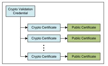
processing rule with a single signature verification action that will accommodate countless public certificates. Certificates can be added and removed from the validation credential independent of any verification actions that use it.
