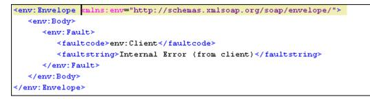
The returned error message indicates that an internal error occurred but no other details are provided. This is by design to prevent malicious attackers from gaining detailed information about the underlying service. You can see detailed information about the failure in the DataPower log.
