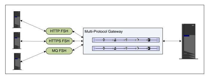
The server-side protocol is completely independent of the front-side and can be any of the protocols supported by the appliance.
