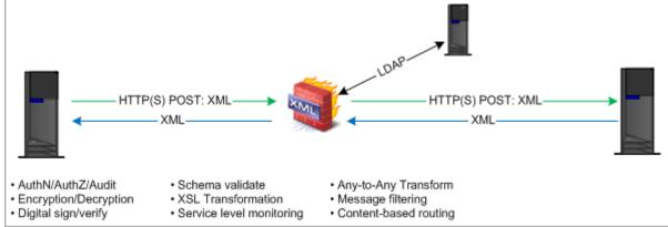
Processing policies have access to all HTTP related details (headers, form fields, payload, status, etc.) for both the request and the response and can therefore make decisions or process messages based on the header's existence or contents.
