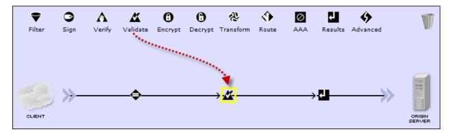
\_\_4. Double click the new validate action (outlined in yellow) to provide the missing configuration details.
