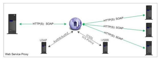
The Web Service Proxy will automatically apply schema validation to both inbound and outbound messages, further assuring message validity. Processing and security policies can be applied not only at the entire service level, but for individual operations within the service as well.
