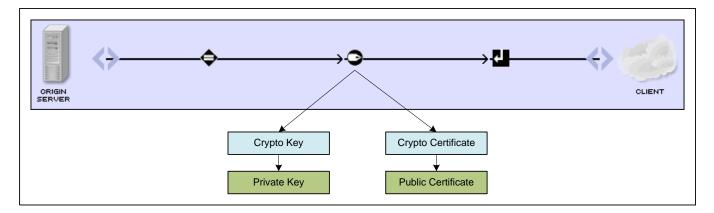
This single level of indirection allows the underlying key or certificate to be replaced without the need to reconfigure any services that are using it.
